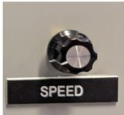
A 10 turn potentiometer precisely controls carrier belt speed to a fixed setpoint. The operator must adjust to match the conveyor speed.
