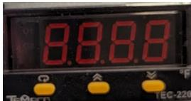
The Watlow 935 or Tempco 220 heat controller precisely controls the air temperature of the heat manifolds. To change the setpoint, press the set button along with the up and down arrows.
